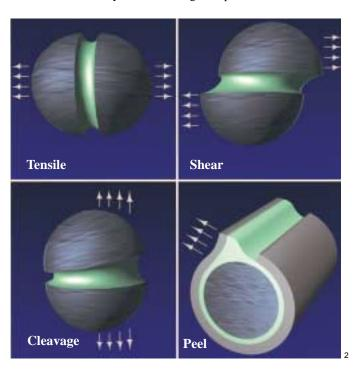
**Tensile** is pull exerted equally over the entire joint. Pull direction is straight and away from the adhesive bond.
